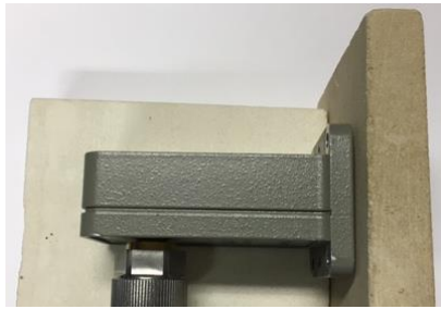
Open Ended Waveguide (OEW)
