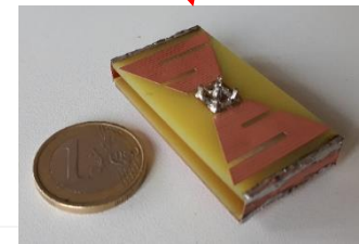
16 cavity-backed antennas with slotted bowtie-like structure
