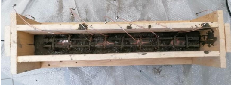
Fig. View of the four SRRs embedded in the mold.
