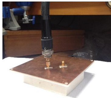
Patch Resonator (PR)
